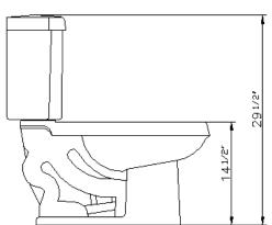
THIS FIXTURE QUALIFIES ACCORD-ING TO ASME TEST PROCEDURES AS A LOW CONSUMPTION WATER CLOSET WITH AN AVERAGE CON-SUMPTION OF 1.6 gpf (6 Lpf) OR LESS.
